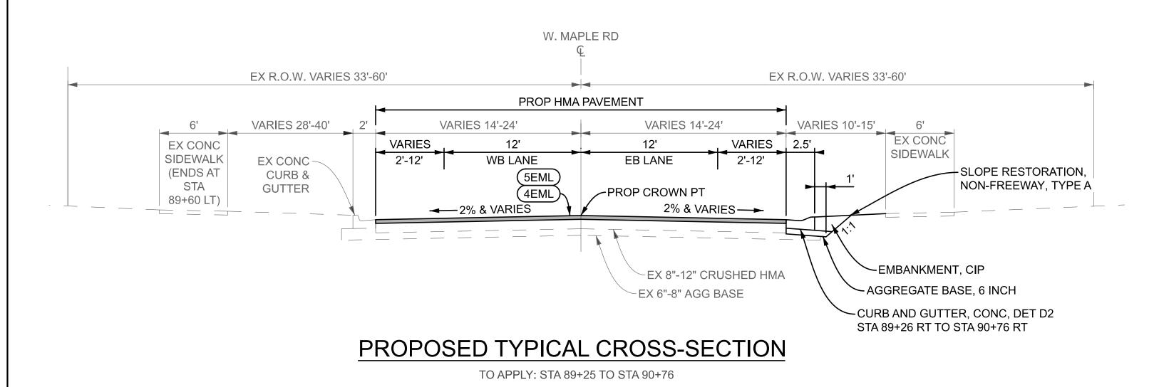
NOTE: FOR "SLOPE RESTORATION, NON-FREEWAY, TYPE A", USE SEED MIXTURE "THM" PER SECTION 816 OF MDOT STANDARD SPECIFICATIONS FOR CONSTRUCTION.
