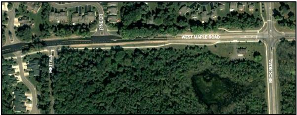
At the time of our field work, the road surface of West Maple Road was HMA paved. The HMA surface was generally observed to be in poor condition, with frequent block cracking and occasional alligator cracking. Frequent pothole patches were observed particularly in wheel paths near the edges of the pavement.
