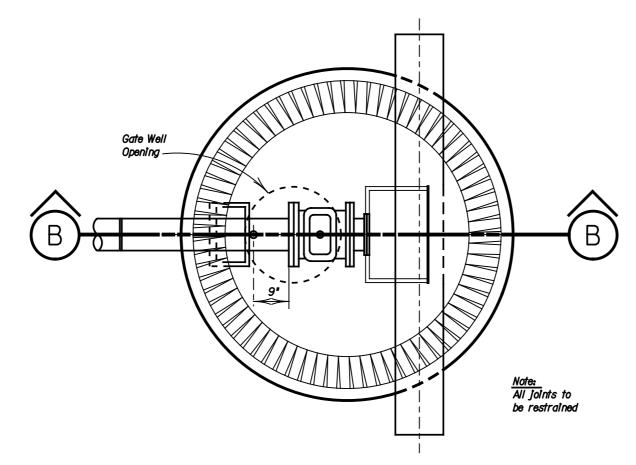
PLAN OF TAPPING SLEEVE, VALVE & WELL
